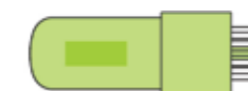
f) side window Matches exit slit, for example, of prism/grating monochromator. The photocathode, is a reflective type located within the glass envelope. Application: Spectrophotometers and photometers.
